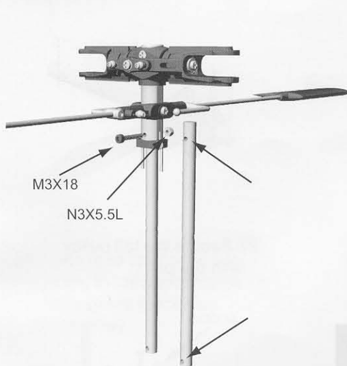
19. Install the main mast. (Be sure not to install the mast up side down)
